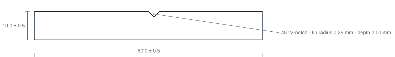
Fig. 3 ISO 179-1 Charpy notched specimen 80 \times 10 \times 4 mm, 45° V-notch, depth 2.0 mm
